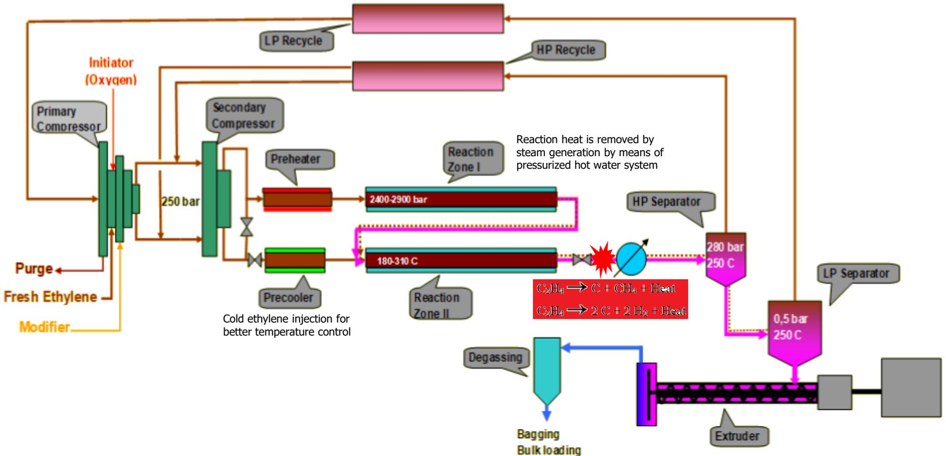
At reaction pressure and temperature LDPE is dissolved in ethylene gas, decreasing the pressure by means of kick-valve will break the homogeneity, expansion increases the temperature of the mixture, cooling is needed to avoid polymer degradation and decomposition of ethylene
