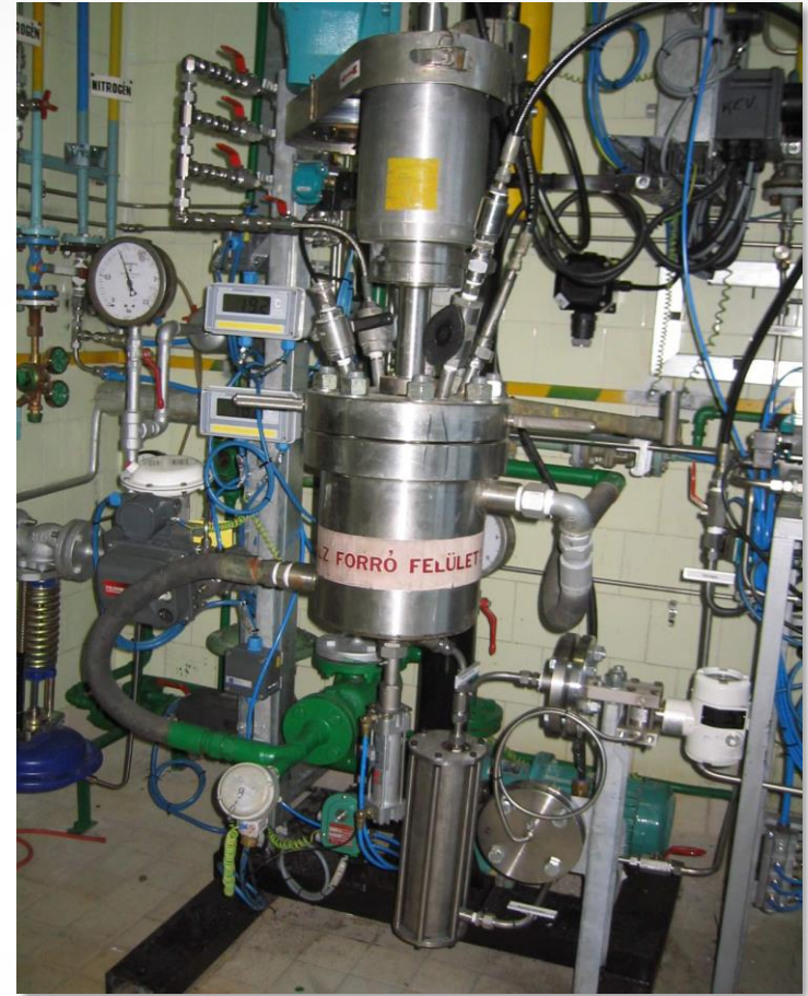
Reactor II. (for HDPE2 and PP cat.)
