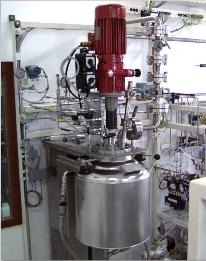
Reactor I. (for HDPE1 catalyst)
