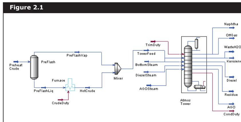
The crude column consists of a refluxed absorber with three side strippers and three cooled pump around circuits. The column sub-
