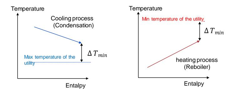
The temperature demand of the utility stream is determined by the level of the condenser and reboiling temperature.
