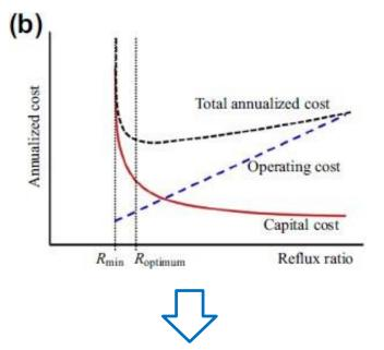
For different numbers of stages, different reflux ratios will be required, corresponding to <u>different reboiler and</u> <u>condenser duties.</u> There is a trade-off between operating costs and capital investment - increasing the number of stages would increase the height of the column and therefore its cost, but would decrease reflux requirements and hence reduce duties and operating costs, as well as costs of heat transfer equipment.
