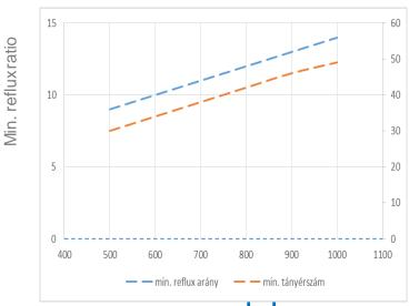
Minimum reflux ratio and minimum number of stages both increase with pressure. With a higher operating pressure, the <u>capital cost of</u> the column will increase.
