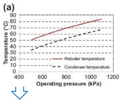
distillation operating pressure affects the temperatures of heating and cooling. The bubble point and dew point temperatures of a mixture of a given composition depend strongly on pressure.
