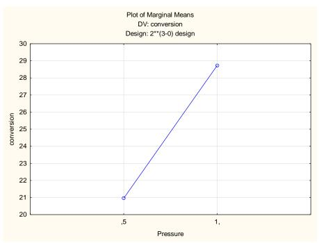
The conversion is higher at higher pressure. If the pressure is increased from 0.5 bar to 1 bar the conversion increases with 3.89%.
