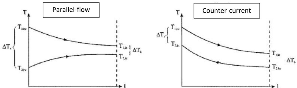
Temperature profile when one of the streams undergoes phase transition during the heat transfer (for example the condensation of a heating steam):
