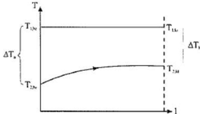
In this case, it makes no sense to talk about parallel flow or counter flow.
